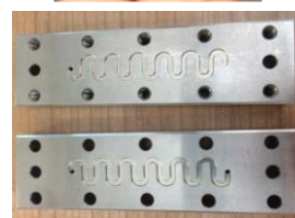
Channel Ø: 800-1000 µm V int : up to 10+mL
