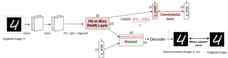
Graphical representation of the structure of our new network, named HitNet. Our contributions are highlighted in red, and comprise a new Hit-or-Miss layer, a centripetal loss, prototypes that can be built with the decoder, and ghost capsules that can be embedded in the HoM layer.
